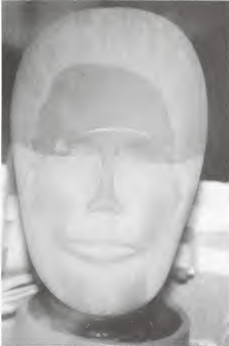
FIGURE 21 -- Frontal View of Chalk Removal Pattern for System I
